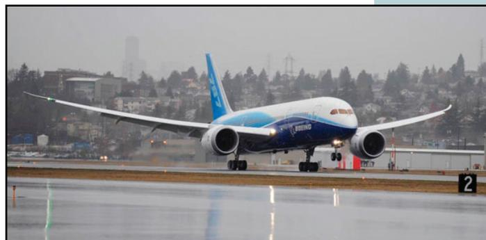
Boeing 787 landing at the end of its maiden flight, illustrating the flexibility of its wings.
